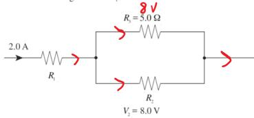
What is the current flowing through the  $5.0 \Omega$  resistor?
