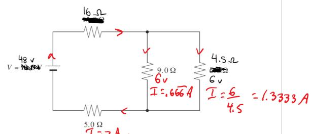
a) Find the power loss through the 5  $\Omega$  resistor.
