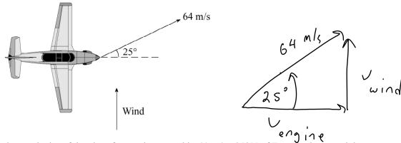
The resultant velocity of the aircraft over the ground is 64 m/s, 25°N of E . At what speed does the wind blow?
