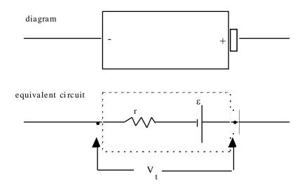
supply Vt = I = current through cell r = internal resistance of the cell  $\epsilon = internal/chemistry voltage (sometimes called emf)$   $V_t = external/net/terminal voltage$ •=battery terminal
