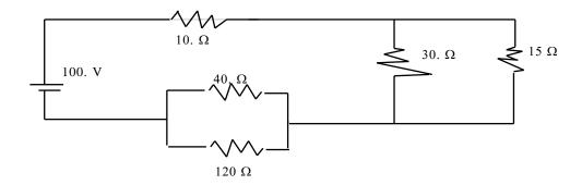
10. Find the cell voltage given that 2.00A flows through the 15.0 $\Omega$ . (225V)
