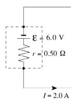
What will be the reading on a voltmeter connected to the battery terminals?
