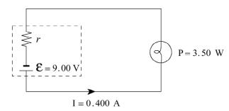
a) If a current of 0.400 A leaves the battery, what is the internal resistance, r, of the battery? (5 marks)
