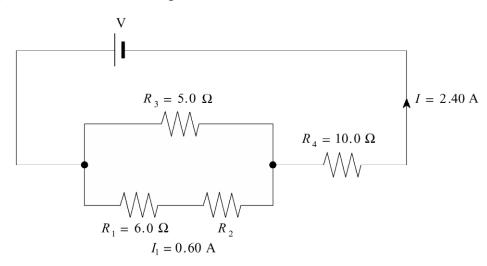
b) Find the potential difference of the power supply,  $V_{\cdot}$
