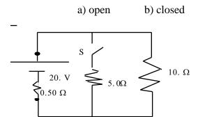
8. find the total current in this circuit when the switch(S) is
