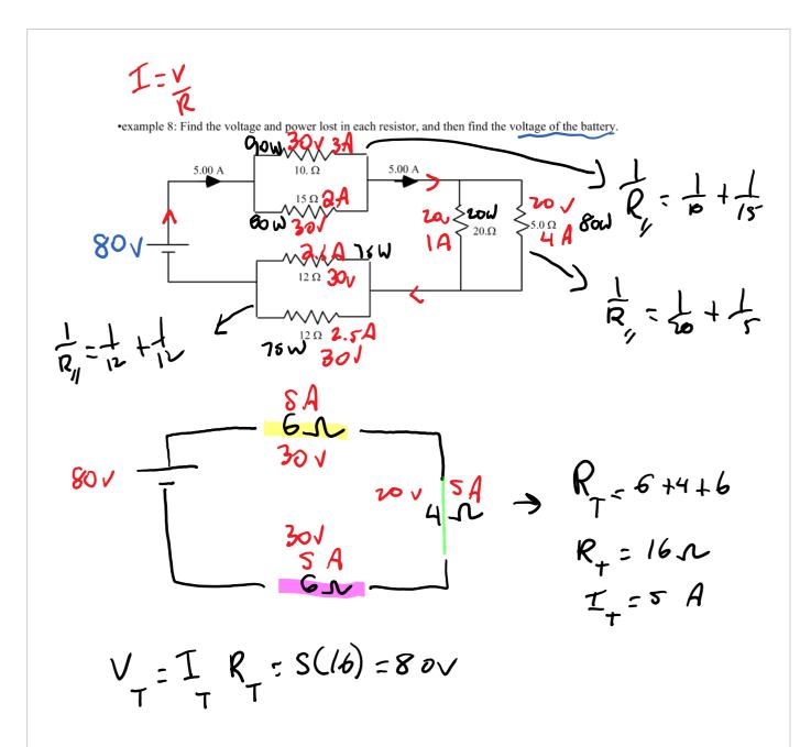
• example 8 illustrates an important point. It shows us that the voltage drop across parallel resistors is the same as the drop across the equivalent resistor in the equivalent circuit.
