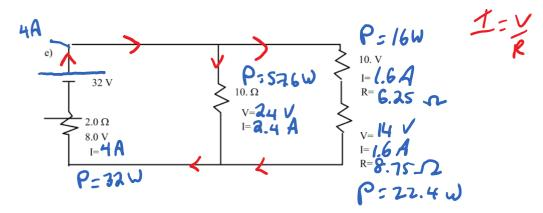
•Lightbulb questions are a good test of student understanding of Kirchhoff's Laws. The brightness of a light bulb is related to the power use (J/s), and therefore depends on the current through a resistor and the voltage drop across the resistor (P=VI)
