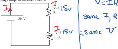
b) if the resistances are not the same then what can we say about the division of the voltage? For instance compare the unknown voltage drops  $V_1$  and  $V_2$  below
