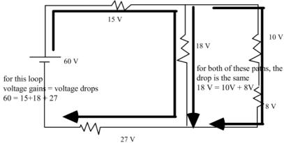
•to see the voltage relationships, it is sometimes helpful (at first) to redraw the circuit so that all resistors are pointing 'downhill'. For instance consider the previous circuit 5a)
