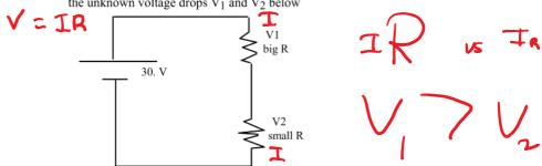
c) if the resistors are simple ratios of each other, we can relate the voltage drops via the same ratios. For instance, find the unknown voltage drops below. (note the first resistor is twice the second)
