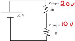
•Although it is helpful at first to label voltages at each point in the circuit, it is desirable at this point to label only the gains and drops. In all of the following examples, the voltages written next to resistors are understood to be the voltage drops. Likewise the voltage numbers written next to cells are the voltage gains.
