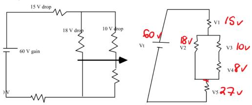
•example 6: write equations relating the voltage drops Vt. V1.V2.V3.V4. V5 in the above circuits
