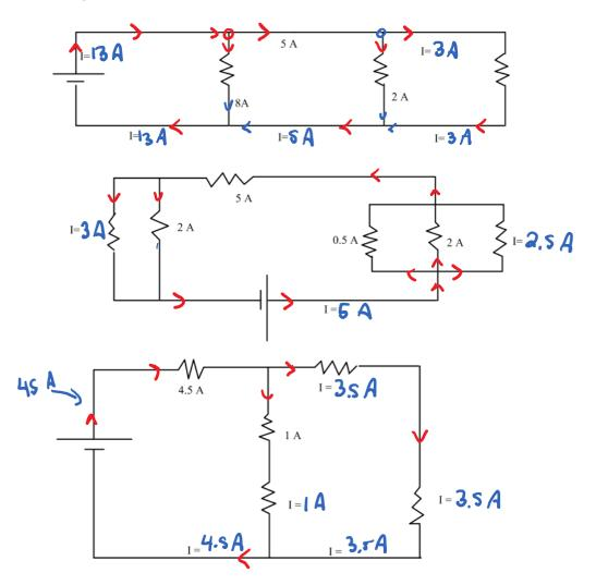
•The amount of flow along a particular path from a junction depends on the resistance of that path.
