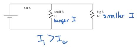
c) if the resistors are simple ratios of each other, we can relate the currents via the same ratios. For instance, find the unknown currents below. (note the second resistor is twice the first)
