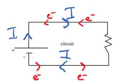
a) electron flow red b) current (conventional current)
