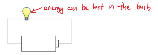
So, electrons need a completed circuit for current to flow!
