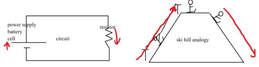
So, potential (or voltage) is like height. Positive charges want to fall downhill in the same way that a ball wants to  $roll\ downhill.\ PE_{grav}\ (mgh)\ is\ like\ PE_{elect}\ (qV).\ The\ only\ reason\ the\ V\ doesn't\ have\ a\ constant\ like\ "g"\ in\ front\ of\ it$ is due to how we defined the volt.  $mgh \sim qV$
