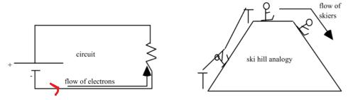
•One problem we encounter with this analogy is that in the circuit, is that it is electrons that flow, from the lower voltage (-) terminal through the wire to the higher voltage (+) terminal.
